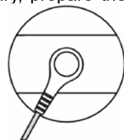
Fig. 1. Way of leadwire and electrode connection
